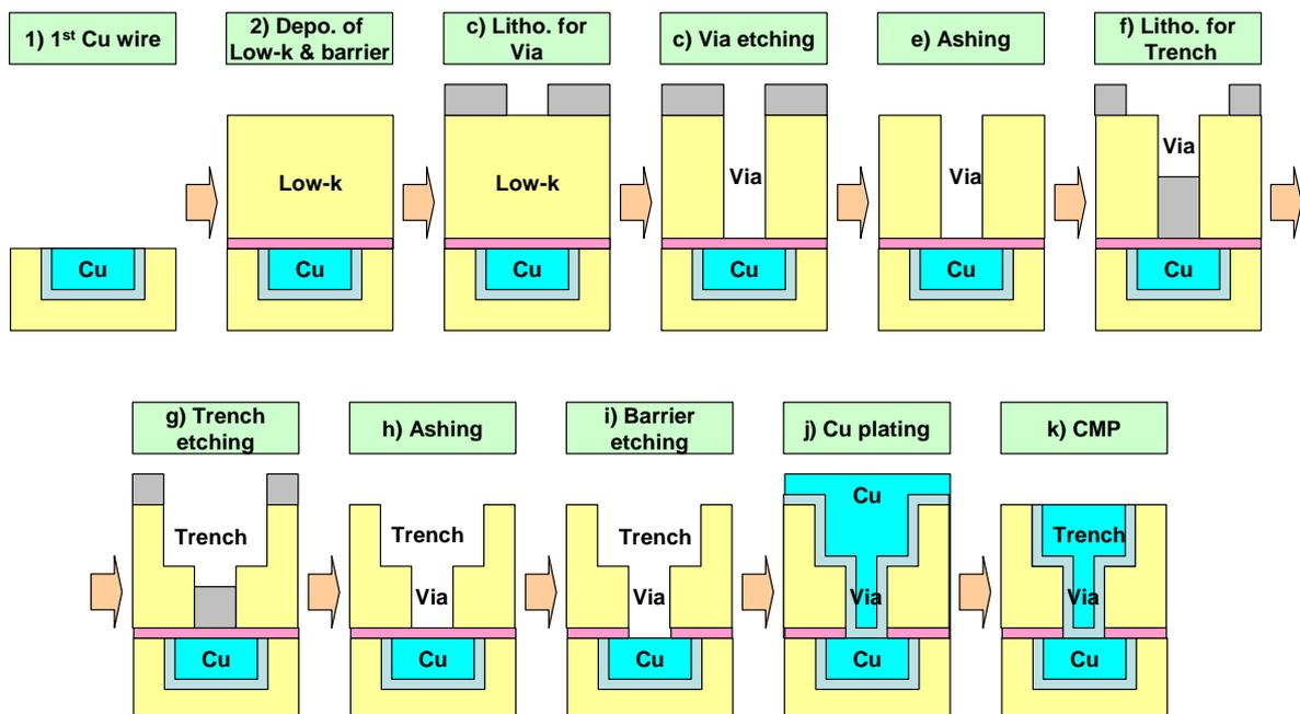
Fig.11 Dual-damascene process flow.
