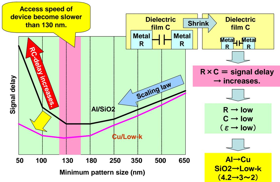
**Fig.9 Cu and low-k film were needed for semiconductor devices.**
