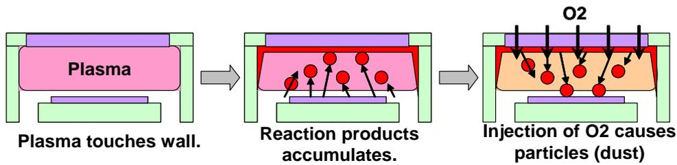
**Fig.13(a) Reaction product control by the conventional oxide etcher in which plasma touches wall.**
