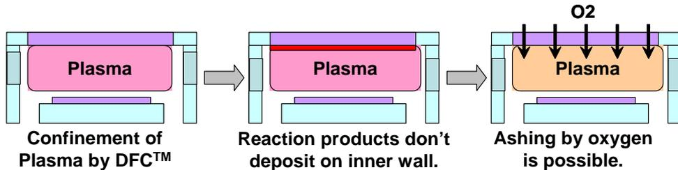
**Fig.13(b) Reaction product control by confinement plasma of Exelan.**
