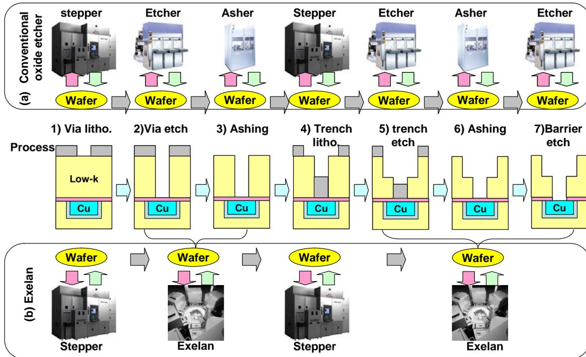
**Fig.14 Dual-damascene by using conventional oxide etcher and Exelan.**
