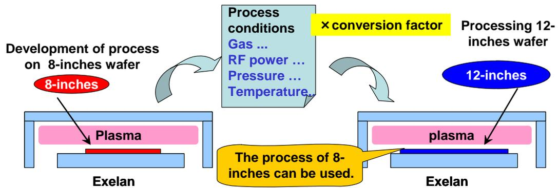
Fig.12 Exelan can etch both 8- and 12-inches wafer.
