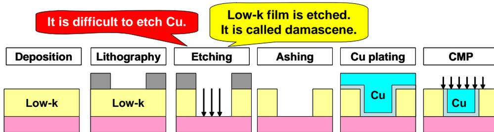
Fig.10(b) Cu/Low-k process.
