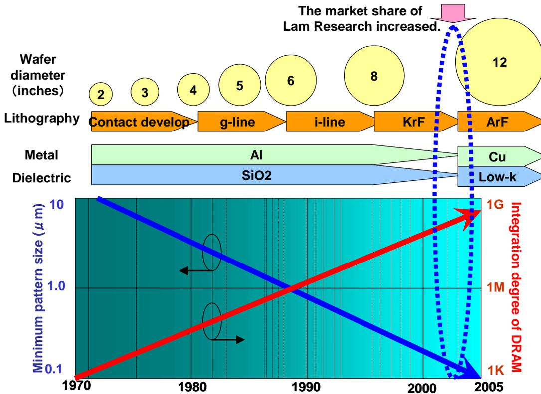
Fig.6 Semiconductor technology in transition.
