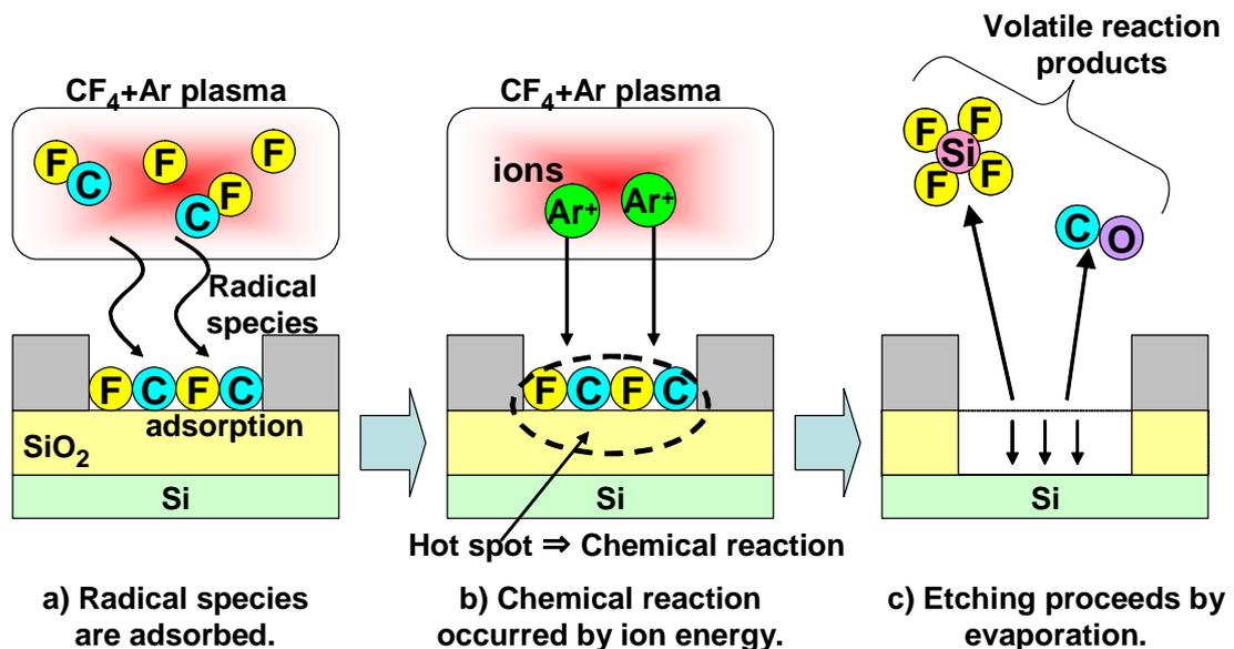
**Fig.5 Mechanism of dry etching (case of  $SiO_2$ ).**
