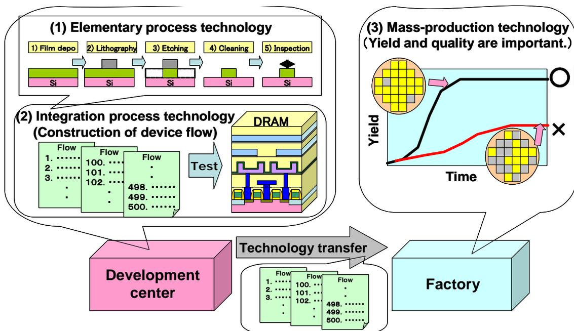
**Fig.1 Three phases of wafer process technology.**
